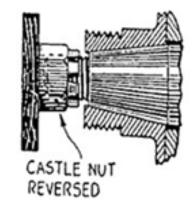
blow. One or two sharp blows on the end of the nut usually will serve to loosen up the tightest wheel with no chance of injuring the threads on the end of the axle,
